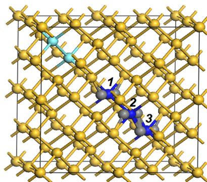
**Figure 2** Supercell (2x2x2) containing divacancy and DIA. Two interstitials are in gray, vacancy in the position of depleted atom is in blue, divacancy is in light blue. Positions 2 (3) correspond to various DIA distances from divacancy.
